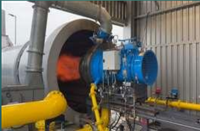
New hydrogen-fuel burner for asphalt production (Photo: Wirtgen Group)
